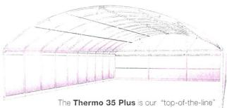
Thermolator. It will hang a full tomato crop and meet building codes. It ventilates better and holds temperatures more stable. It features trussed arches and an 8' eave height. With 4 webs, a set of signed engineered drawings are included with calculations verifying that it meets building codes to 20# live load and 80mph wind loads. With 6 webs it will also hang
