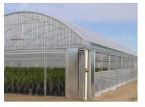
**Natural Ventilation:** Roof vents, wall vents, Roll up Walls, Drop walls.
